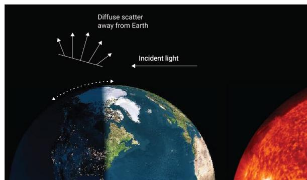
Notably, this off-pointing maneuver results in a 25% reduction in available power for the satellite. Despite this cost, SpaceX has specifically designed the second-generation satellite to be able to accommodate this significant power reduction to minimize brightness as viewed from the ground.
